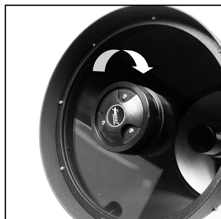
Figure 4-1 Rotate the collimation screw cover to access the three collimation screw.
